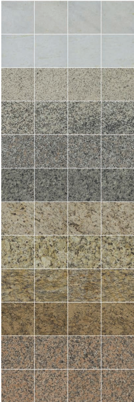
Fig. 5 The dataset of granite textures used in the experiments (unrotated images). From the top: Acquamarina , Azul Capixaba , Bianco Cristal , Bianco Sardo , Rosa Beta , Azul Platino , Giallo Ornamentale , Giallo Napoletano , Giallo Santa Cecilia , Giallo Veneziano , Rosa Porriño A , Rosa Porriño B .
