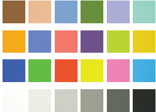
Fig. 10. The 24 colour patches of the x-rite ColorChecker ®.
